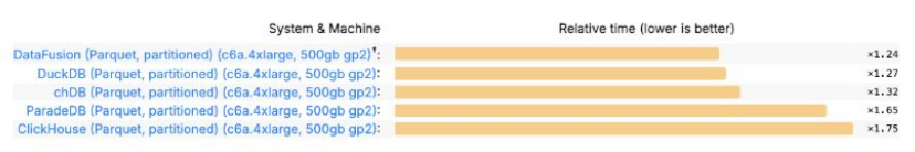
Figure 1: 2024-11-16 ClickBench Results for the 'hot'[ ^ 1] run against the partitioned 14 GB Parquet dataset (100 files, each ~140MB) on a c6a.4xlarge (16 CPU / 32 GB RAM) VM. Measurements are relative (1.x) to results using different hardware.
