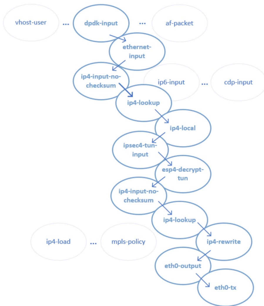
Figure 1. VPP Packet Processing Graph with IPsec-related nodes highlighted
