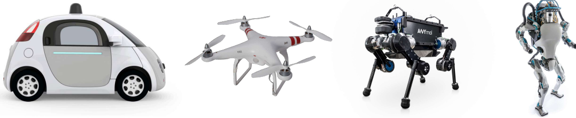
Figure 1.3: Floating-base systems for which the base cannot be directly actuated. Algorithms for the control of self-driving cars [26] and drones [27] are quite mature, whereas those for legged robots, such as quadrupeds [28] or bipeds [29], are still an open research question. The difficulty to control legged systems comes largely from the various restrictions for the creation of external forces.
