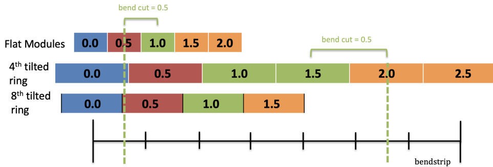
Figure 21: Representation of the encoding and proposed decoding algorithm for three rings in layer 1. Each row shows the encoding of a specific ring and their lengths represent the range in bendstrip that is covered by their stub window size. The half integer numbers are the possible (positive) bends, and the colors represent their mapping to the encoded bend. The green dashed lines represent the decoded bend for an encoded bend of 2. The encoded bend is a representation of the detector bend in 3 bits, an encoded bend of 2 does not correspond to a detector bend of 2. The bend cut is a tunable parameter.
