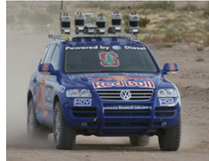
Fig. 1. Stanley, the Stanford Racing Team’s entry in the DARPA Grand Challenge 2005, under autonomous control, with no human in the vehicle.
